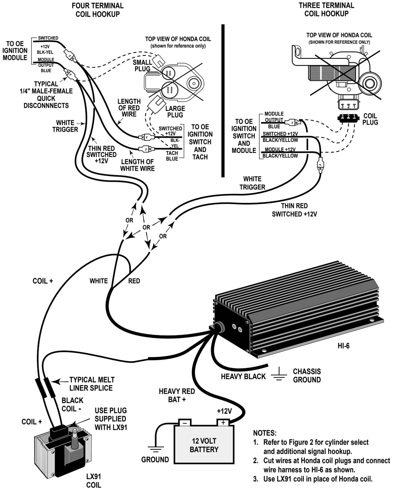
Figure 8. Honda Internal Coil Hookup
